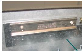
The new MM300 unit is mounted on the DIN rail. No new holes are required in the chassis.
